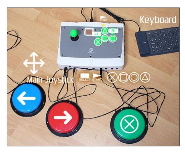
**Top view: C-SID** with three Able-net accessibility switches attached and roll-up keyboard (not supplied).
