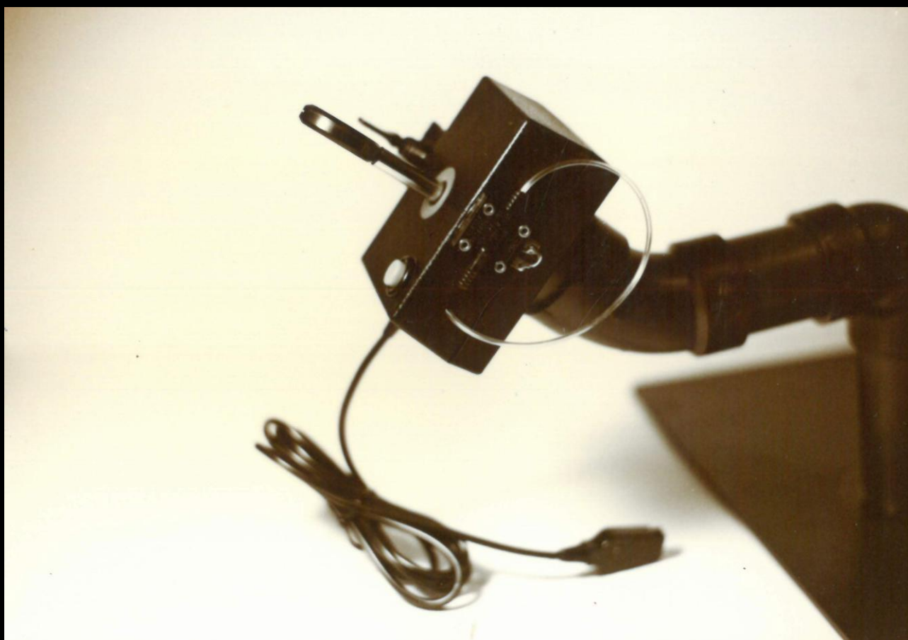
Model 103: Mouth operated controller for quads.
