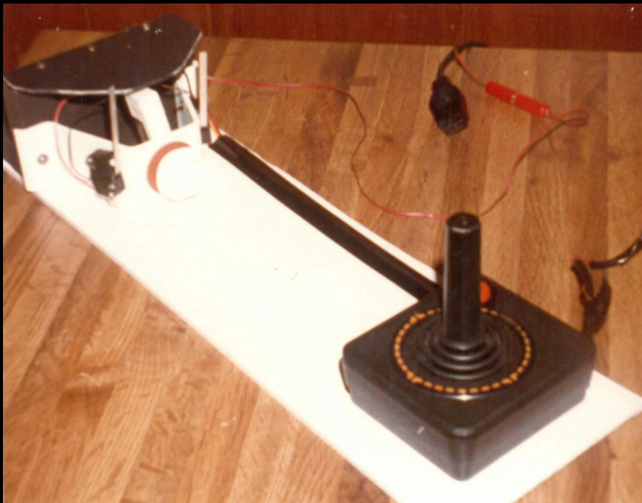
Custom CX40 joystick with fire button hooked up for limb control.
