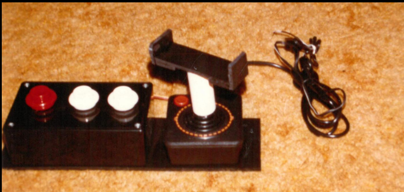
Model 107 derivative, modified joystick with slip on crade and three soft touch buttons.
