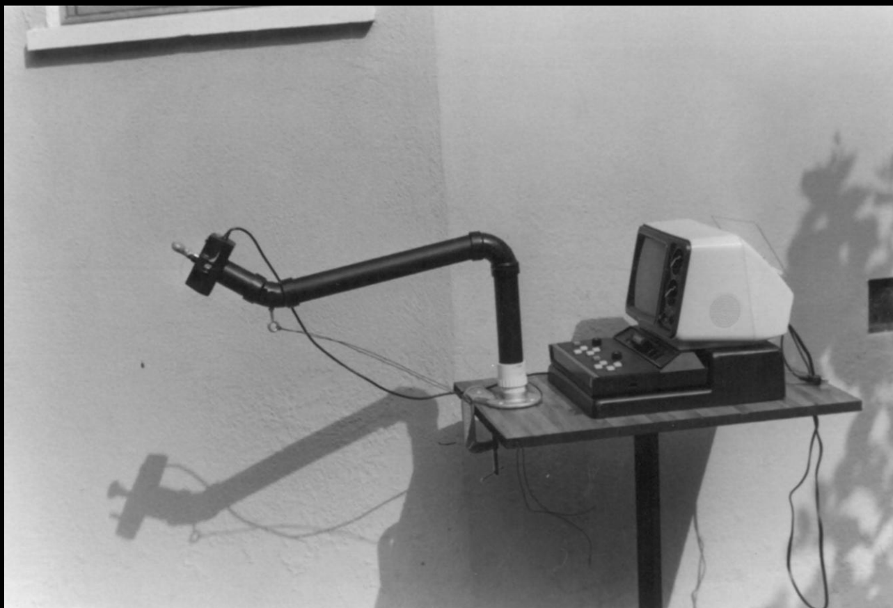
Model 103 Mouth controller on long PVC piping mount plus Model 403 video game unit.
