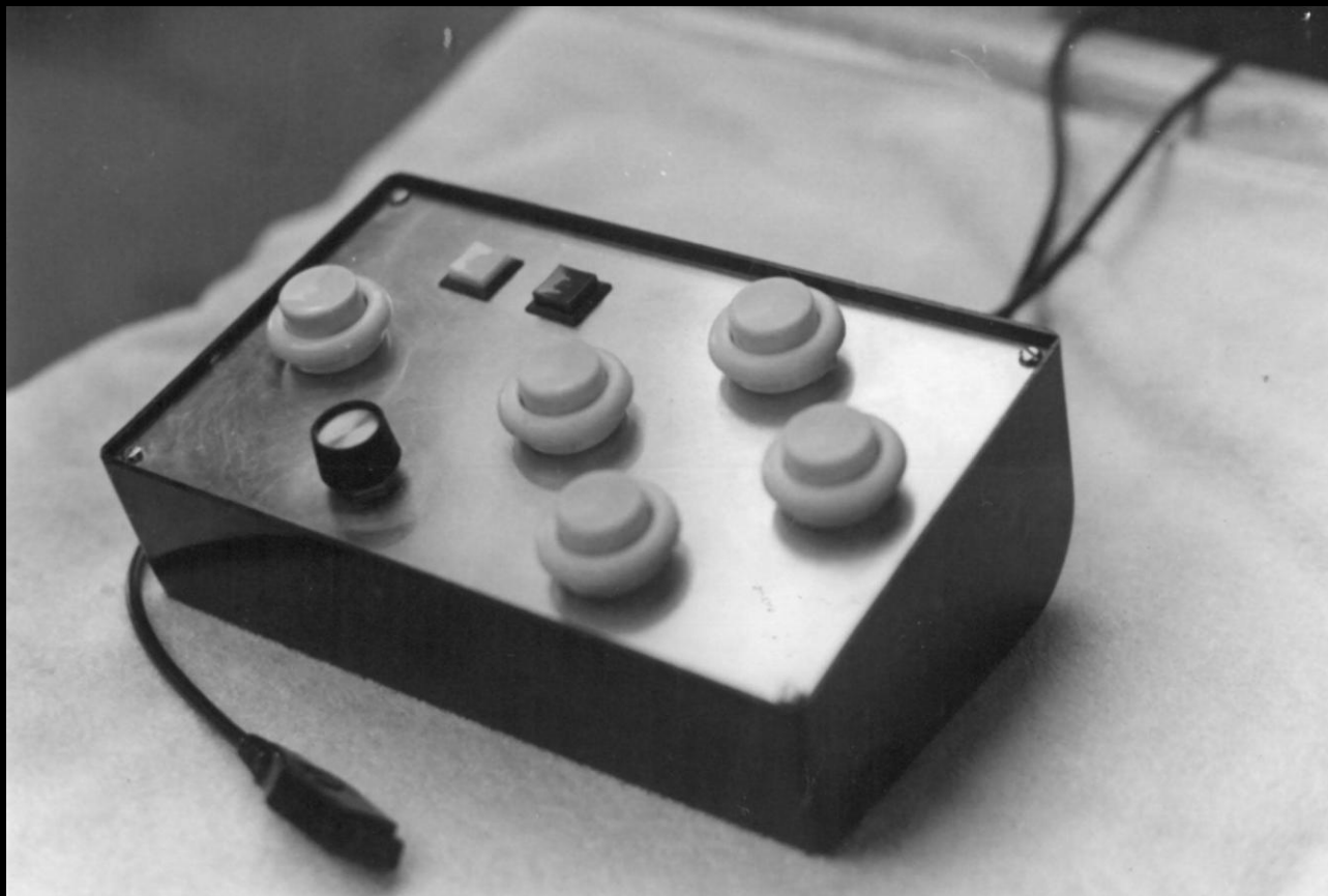
Model 102: Hand / wrist controller with paddle and select and reset buttons.
