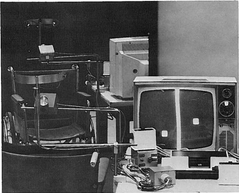
**FIGURE 4.**—Odyssey game with external modifications. Shown is a chin bracket with chin control on horizontal bar.
