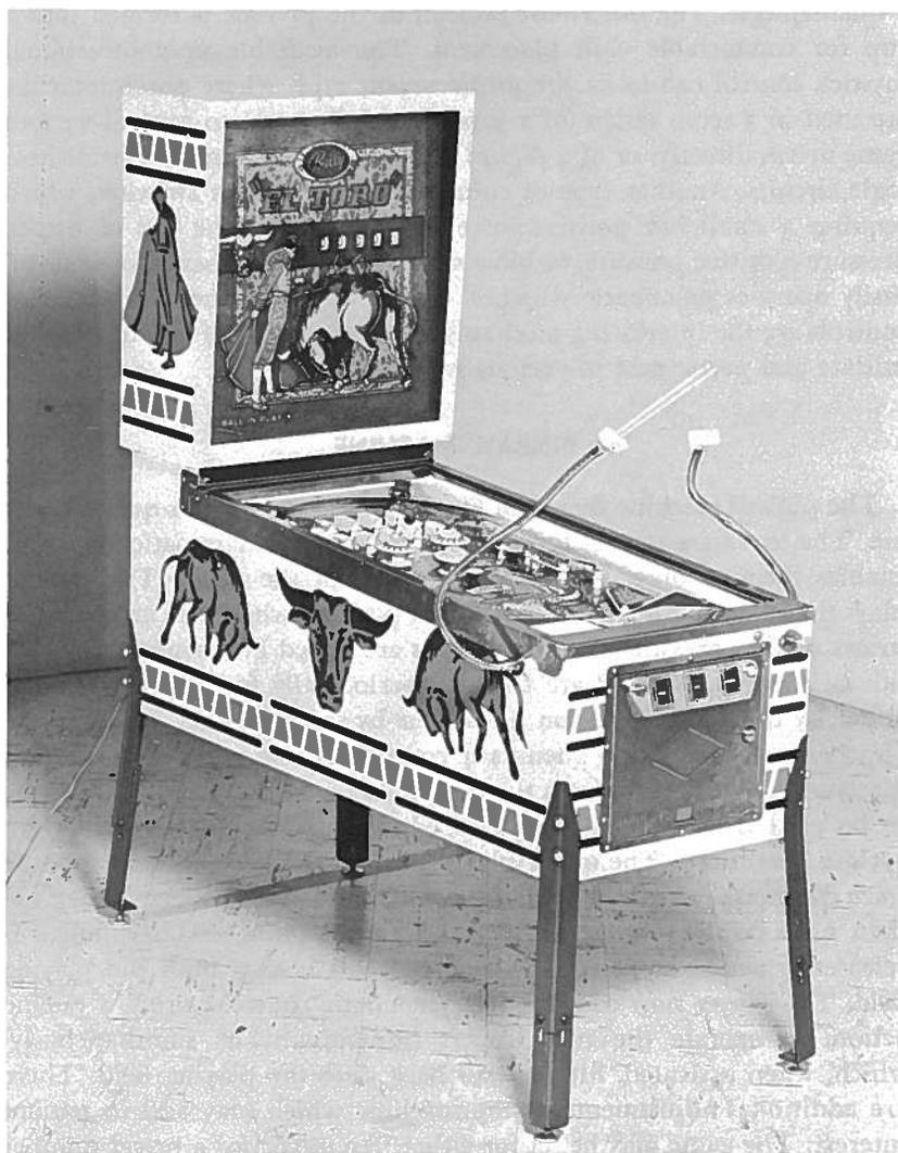
FIGURE 1.—Pinball game, modified for quadriplegics, with pneumatic controls and slotted adjustable legs.
