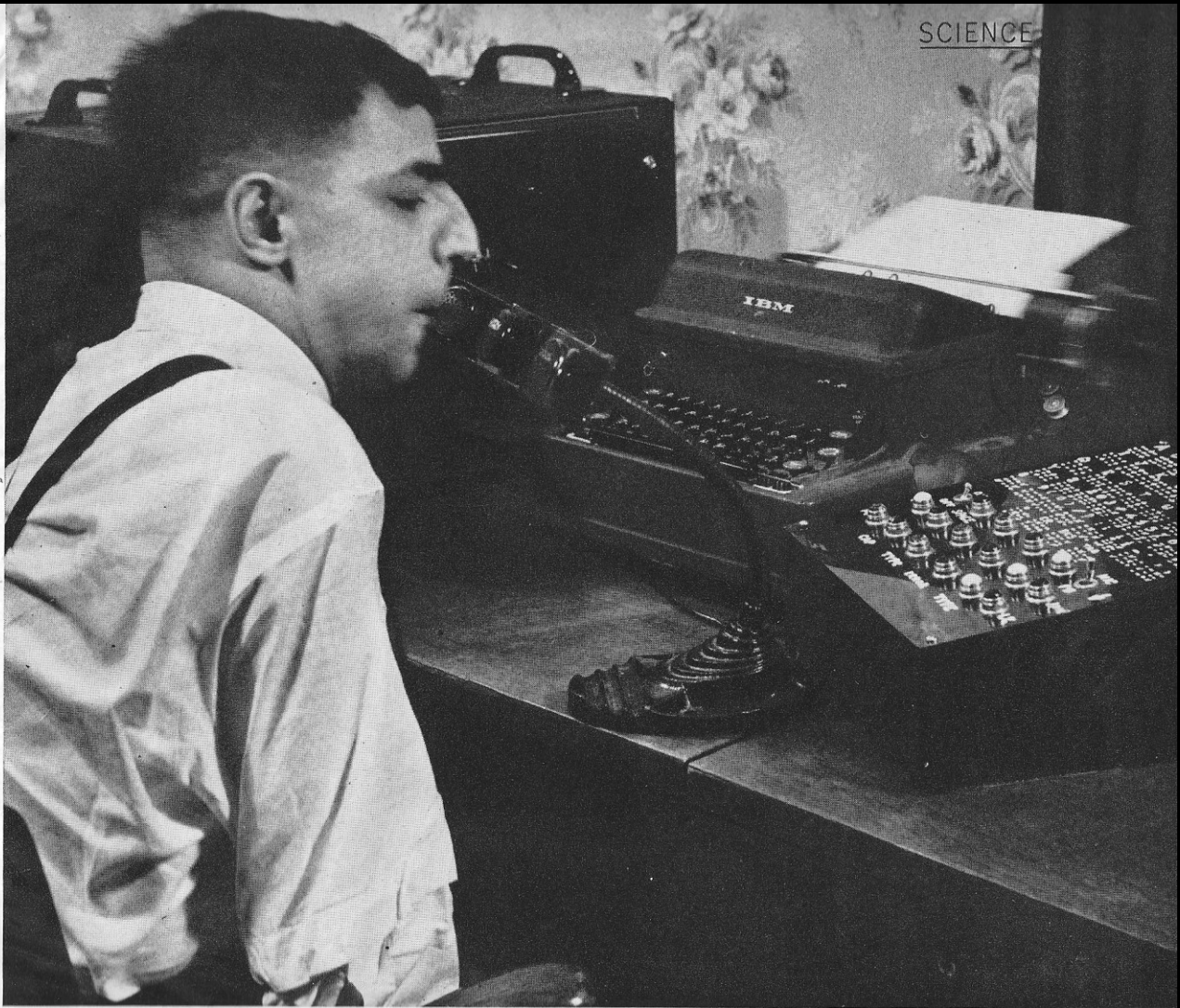
AVAKIAN BLOWS INTO MIKE TO WORK HIS TYPEWRITER. ELECTRIC IMPULSES FROM MIKE GO THROUGH CONTROL BOX (RIGHT) AND ELECTRONIC BRAIN (LEFT)
