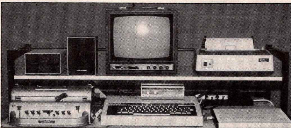
Above: the Computing and the Blind project at the Open University has made tremendous progress; people like David can use this workstation to produce normal and braille hard copy. The system includes BBC micro, Perkins Brailler and an embossed overlay which (right) is used with a concept keyboard to provide, in this case, talking arithmetic for young visually handicapped pupils.
