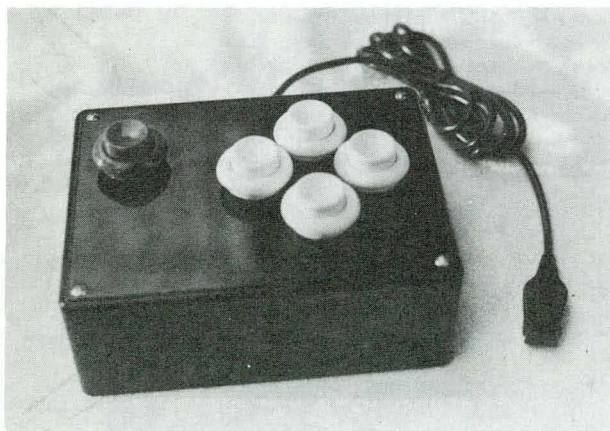
Figure 1. The Finger-Tip Controller, found to be applicable to a wide variety of handicaps.
