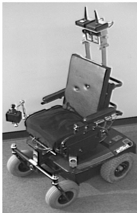
**Figure 4.** Arrow-XT™ configured for VP Control.
