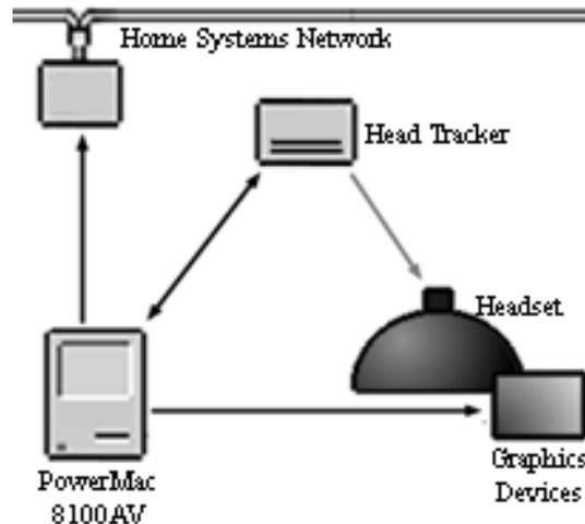
**Figure 2.** System communication schematic
