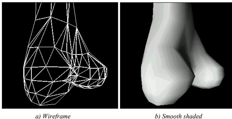
**Figure 5.** *Graphical object display*
