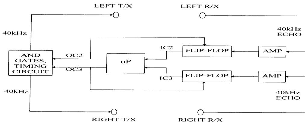
**Figure 2.** Microprocessor control of ultrasonic transmission/reception process
