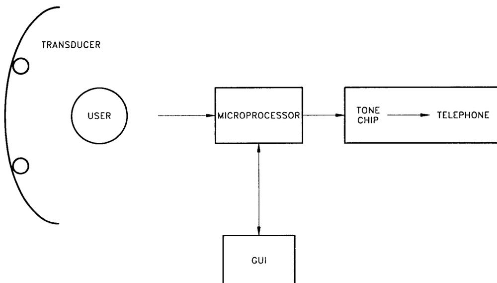
**Figure 3.** Block diagram of the telephone interface
