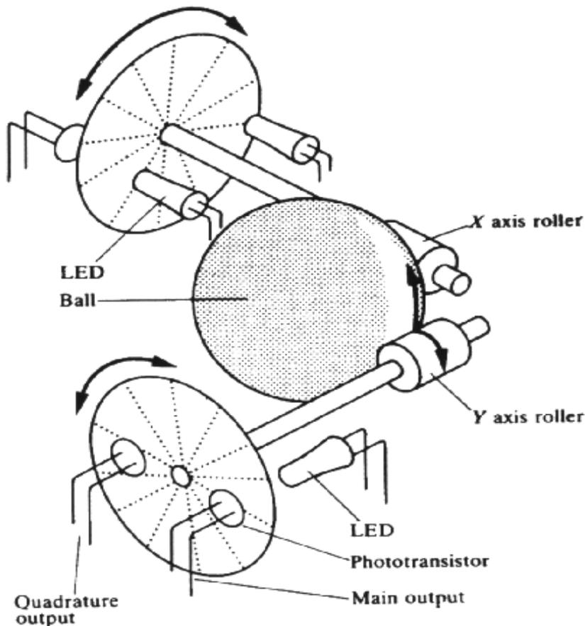
Figure 6. The mechanical system of a mouse
