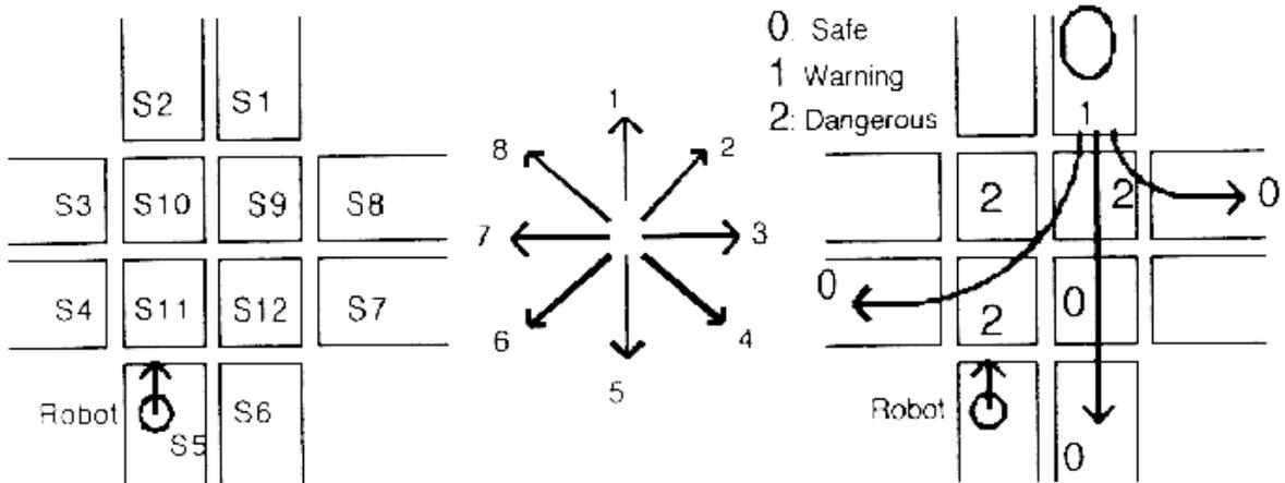
(a) Sections at the cross (b) Quantized directions (c) Danger estimation for a front vehicle
