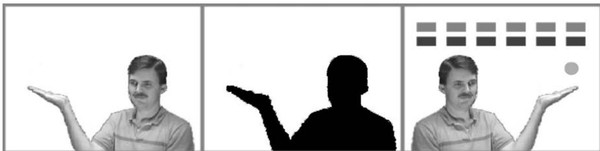
**Figure 3.** Example images at various points in the Virtual Interaction system. The left image is typical of the camera output. The center image is the user's silhouette, as produced by the chromakey. This is the image that the system reacts to. The image on the right is the resulting image shown to the user.
