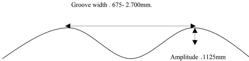
**Figure 3.** *Profile of grooved sinusoidal texture*
