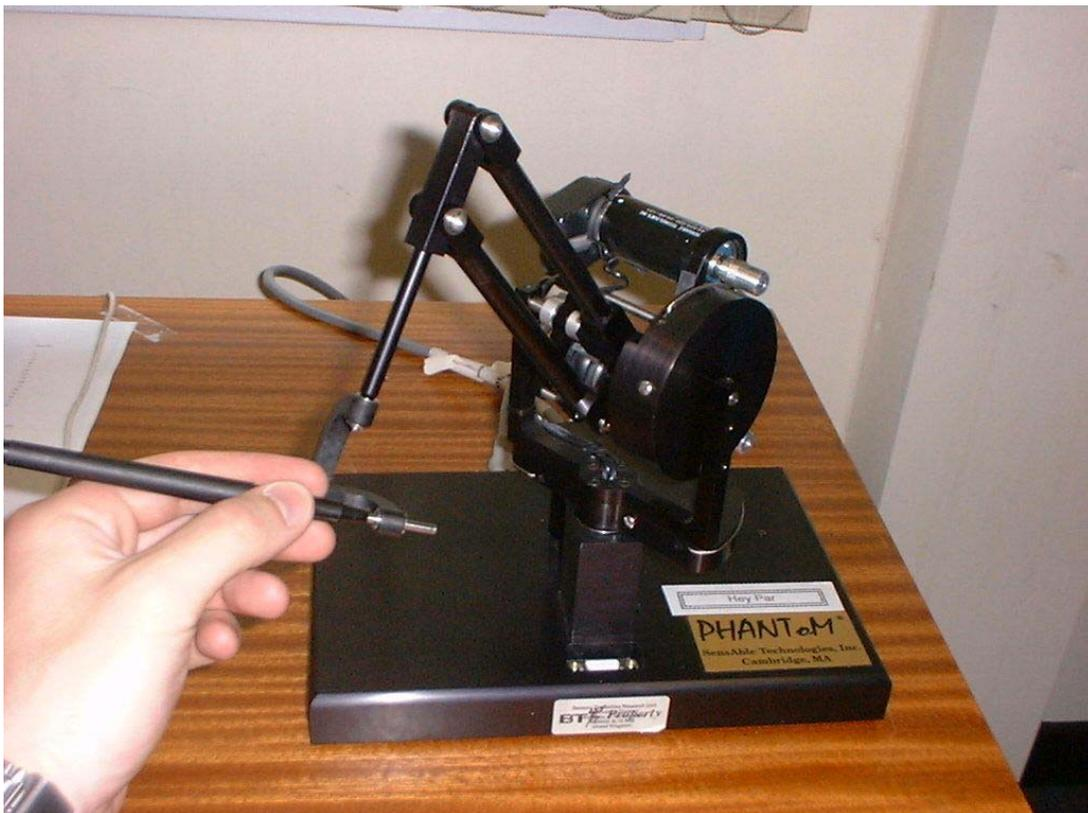
**Figure 2.** *The PHANTOM 1.0 with stylus interaction device*
