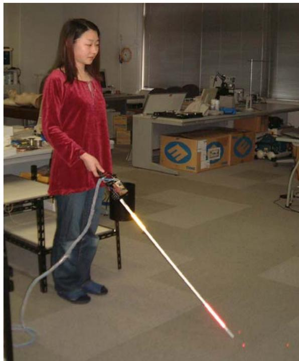
**Figure 2.** *The prototype of Intelligent Cane.*
