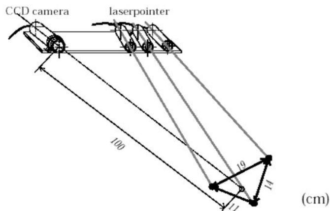
Figure 3. The design of active-stereo range sensor
