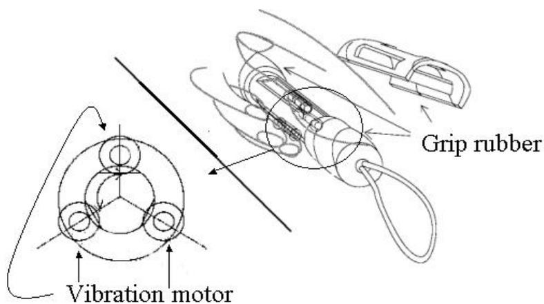
Figure 4. The design of tactile display
