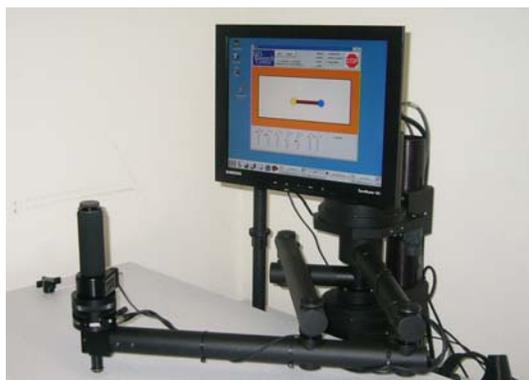
**Figure 1.** *InMotion2 Robot with graphic display of virtual beam task.*
