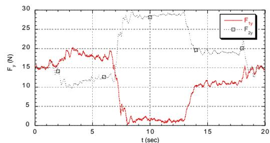
**Figure 12.** Vertical force applied in zero delay test.
