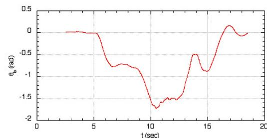
**Figure 15.** Beam angle for 0.5 sec time delay test.
