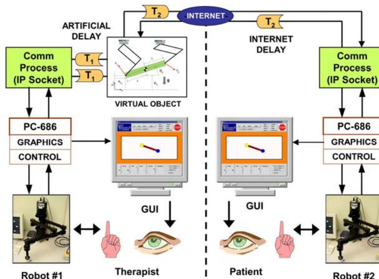
Figure 4. Hardware configuration for Cooperative Rehabilitation Mode.
