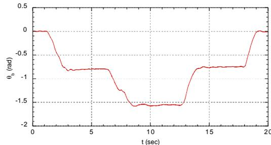
**Figure 11.** Beam angle for zero time-delay test.
