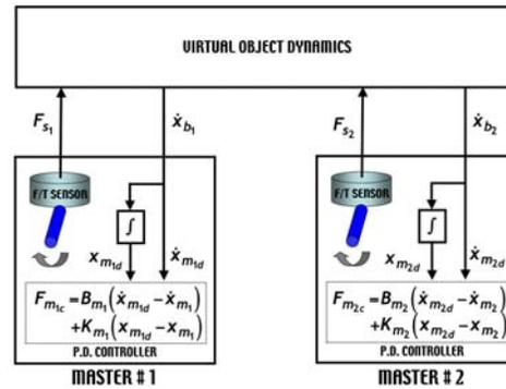
The haptic controller works well for the interconnected robot configurations shown in Figures 3 and 4 as long as the roundtrip time delay is under about 100 msec. As the time delay starts to exceed 100 msec, the passivity of the controller becomes severely compromised and can drive the system unstable. To restore passivity in the system, compensation using wave variables emerged as the most natural approach for performing cooperative tasks over the internet (Niemeyer and Slotine, 1998).
