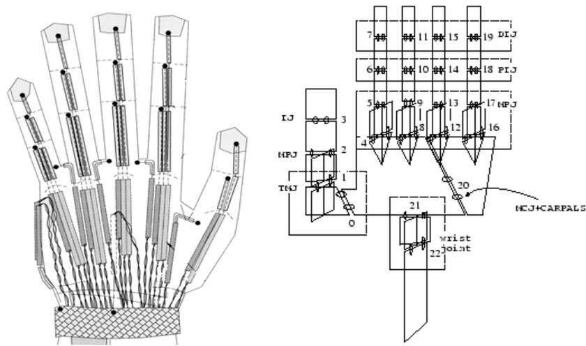
Figure 5. Bend sensor arrangement and target hand model.
