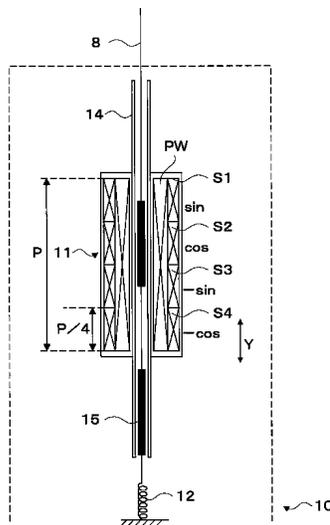
Figure 3. Detailed design of Inductocoder.
