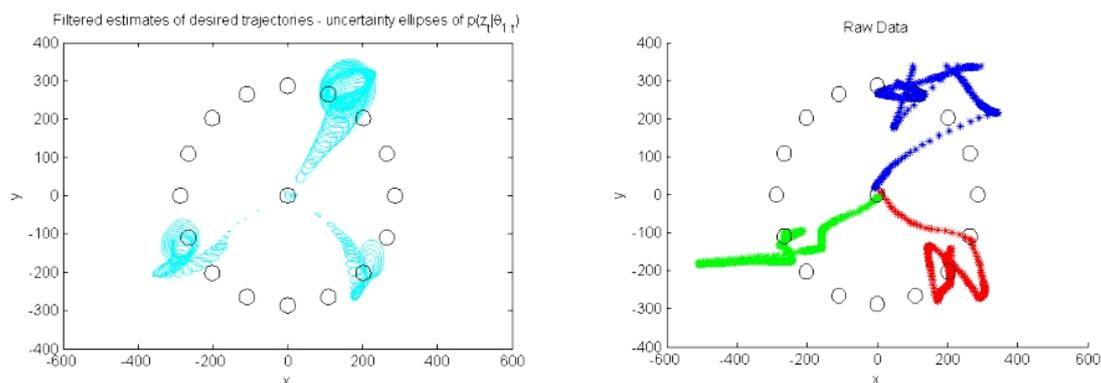
**Figure 3.** Left hand side: filtered traces, showing confidence ellipses obtained from the sequential Monte Carlo filter. Right hand side: corresponding noisy trace data. Note that the filter has 'smoothed' much of the erratic jumping behaviour and quite clearly identified the user's intended destination, despite the ambiguity of the data.
