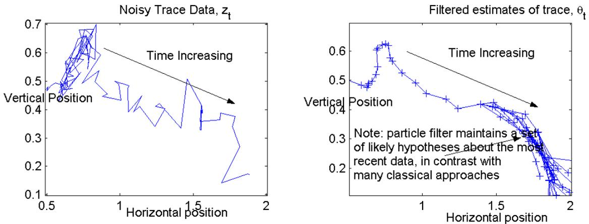
**Figure 2.** Left hand side: Noisy trace data  $z_t$ , generated from a near-constant velocity model in Gaussian noise (range/bearing domain). Right hand side: estimated paths  $\theta_t$  using variable rate particle filter. (Godsill04b). Note the models automatically adapt in the presence of ‘tremor’ like behaviour.
