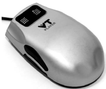
**Figure 2.** *The VTPlayer tactile mouse ([www.virtouch2.com](http://www.virtouch2.com)). The mouse incorporates two, 4-by-4 tactile pin-arrays, on which the index and middle fingers are placed during operation.*
