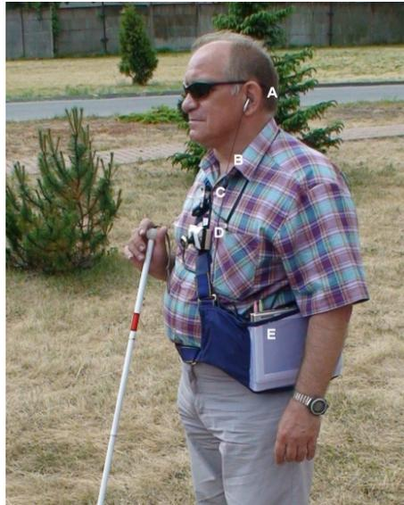
**Figure 1.** Trial participant wearing the prototype for communication with a remote assistant: A – earphone, B - microphone, C – Bluetooth GPS receiver, D – webcam with a fish-eye lens, E – Flybook laptop with built-in UMTS/HSDPA modem and touchscreen.
