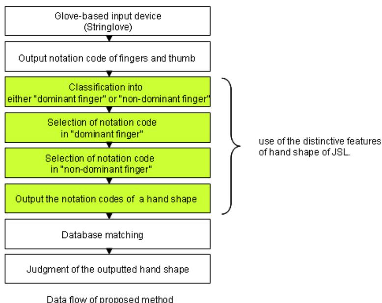
**Figure 2.** Flow chart of proposed method to recognize hand shape with distinctive features.
